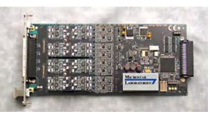
Figure 3 - MSXB 065 signal conditioning board
