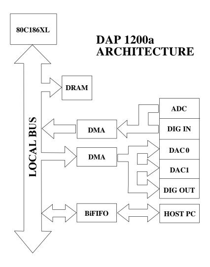
Figure 1: DAP 1200a Data Acquisition Hardware
