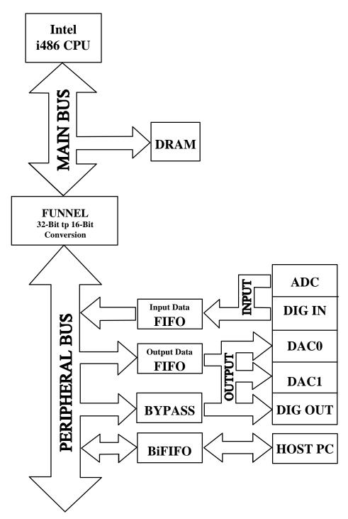
Figure 1: DAP 3216a Data Acquisition Hardware
