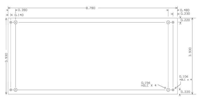
Figure 2. Dimensions of the module
