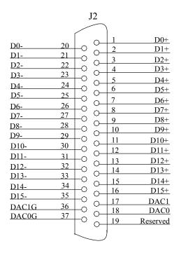
Figure 3. Pinout of the 37-pin input/output connector
