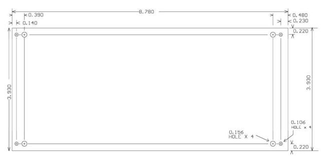
Figure 4. Dimensions of the module
