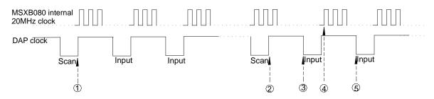
Figure 8. Timing diagram for scan and input addresses
